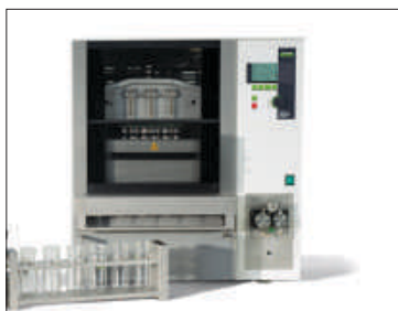
Pressurized solvent extraction with SpeedExtractor
