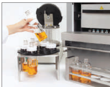
Sample transfer from SpeedExtractor to Multivapor™
